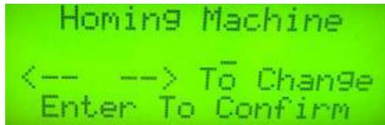
This menu allows you to home the cutter. Homing should be redone anytime the pinch wheel positions have been changed.
