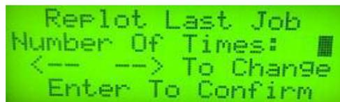
This menu allows you to re-plot the last job up to 999 copies. If the last job plotted was larger than the buffer then a re-plot will not be possible.
