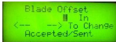
This menu allows you to change the tool offset which is automatically set when you select the tool. You should only change this setting only to improve the corner cutting quality with a dull blade. Note: if you select the tool after changing the offset, the preset offset will take placed.
