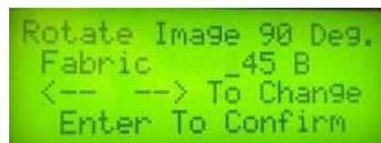
This menu allows you to rotate the job 90 degree. By changing the rotation, cutter will move to the new origin which is upper right corner for 0 degree selection or lower left corner for 90 degree selection.
