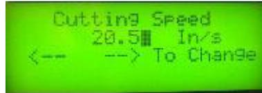
This menu allows you to change the cutting speed of the cutting head between **4-101** centimeters per second (1.6-40 inches per second) for 1062A; and between 4-115 centimeters per second (1.6-45 inches per second). You can change the cutting speed while the cutter is cutting as well as while it is not cutting. Speed settings sent by your computer software may override settings made at the keypad.
