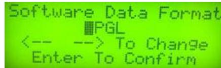
This menu allows you to switch between HPGL (Hewlett Packard Graphic Language) or APDGL (Advanced Plotting Devices Graphic Language). Select HPGL for communication with most of the Sign Software and APDGL for communication with Corel Draw, Microsoft Word, and Adobe Illustrator.
